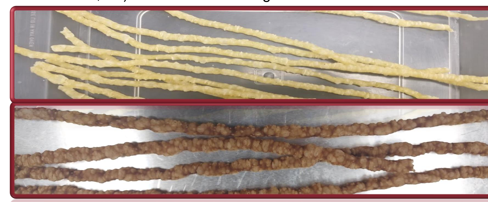
Fig 2. Extrudate with 0% hemp (top insert) and 10% hemp (bottom insert) inclusion into the formula
