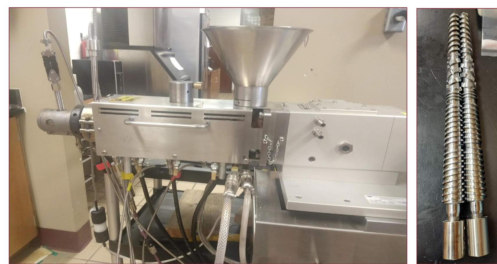
Fig. 1 Lab scale twin screw extruder (C.W. Brabender, South Hackensack, NJ) with counter-rotating twin screws
